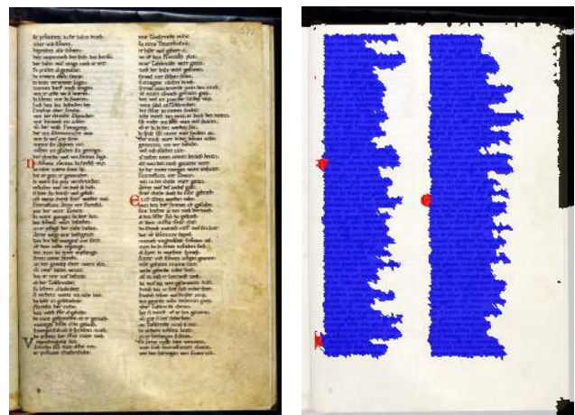
Figure 1: Page segmentation result. The left is the original image. The right is the segmentation result by using the proposed method. The colors: black, white, blue, and red are used to represent: periphery , background , text block , and decoration respectively.
