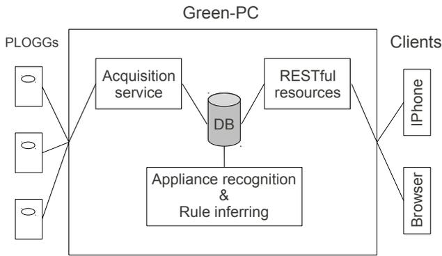
**Fig. 2.** The software architecture of our Green-PC
