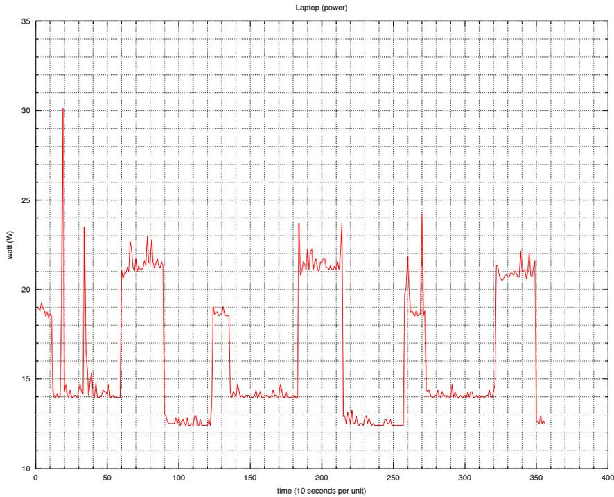
**Fig. 3.** Example of the active power consumption measured for an appliance of class “laptop”
