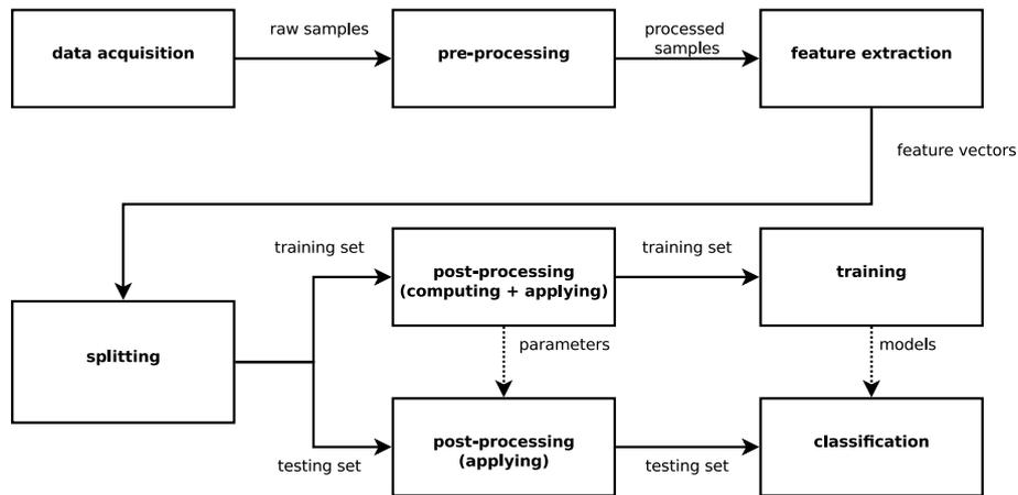
**Fig. 4.** The machine learning process
